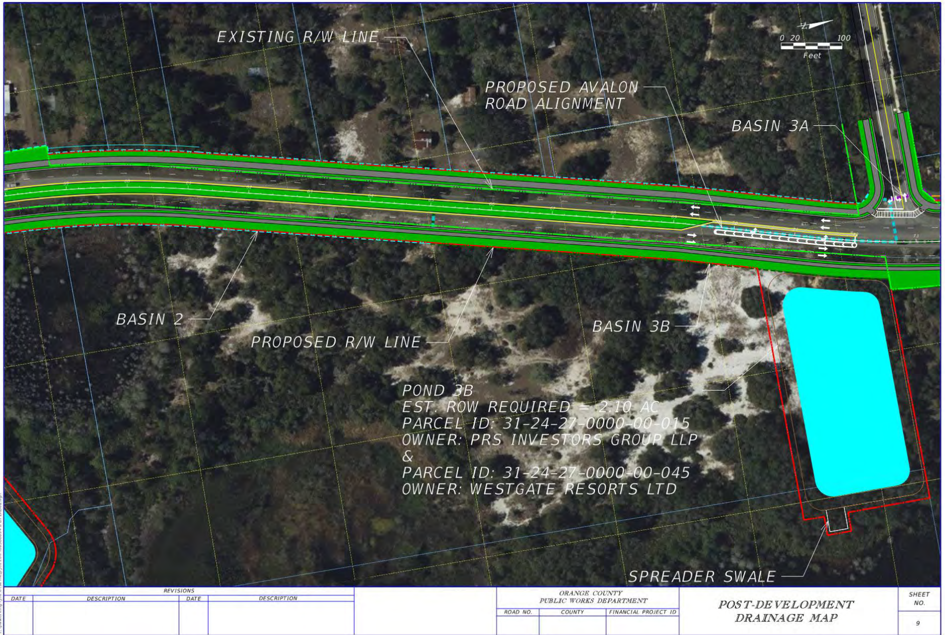
Figure 7-2 – Post Development Drainage Map
